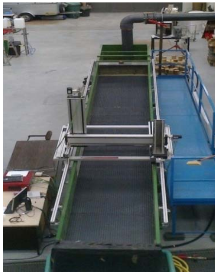
Fig. 1. Open channel flume used in experiments (IMFT, 2015).
