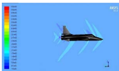
Fig. 5c. Pressure Contours at Mach number 1.5 AoA 0
