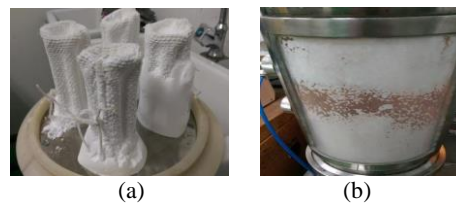
Fig. 4. Problems in fluidized bed granulation process: (a) Particles remained at filter bags (b) Particles adhere to chamber wall.
