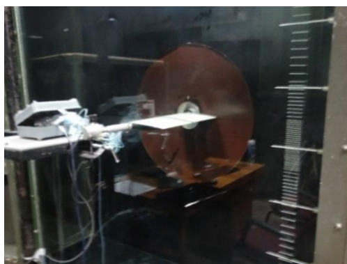
Fig. 3. NACA 0012 airfoil model mounted in the wind tunnel with instrumentation for pressure acquisition.
