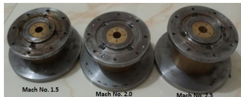
Fig. 6. Fabricated nozzles for Mach numbers 1.5, 2.0 and 2.5.
