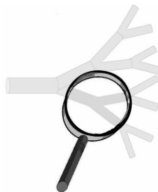
Fig. 1. Schematic representation of a binary-tree-shaped flow network. A parent tube branching into two daughter tubes is the main building block of the tree network of tubes.
