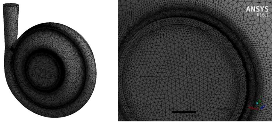
Fig. 3. The mesh structure in flow domain.
