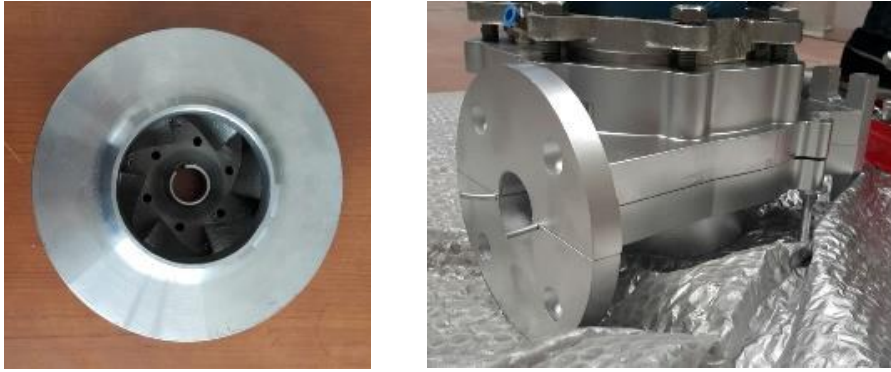
Fig. 5. Impeller and volute manufactured and tested.
