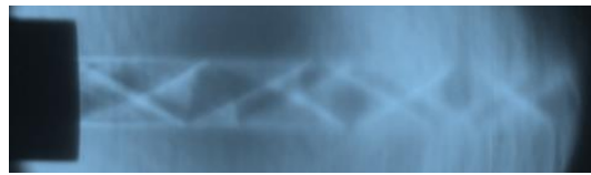
(a) Nozzle controlled with 1.5 mm strut
