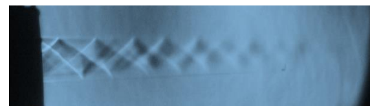
(c) Nozzle controlled with 3.5 mm strut
