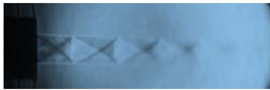
(c) Nozzle controlled with 2.5 mm strut
