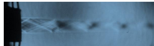
(a) Nozzle controlled with 1.5 mm strut
