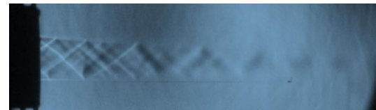
(a) Nozzle controlled with 1.5 mm strut
