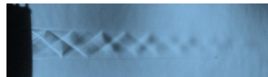
(b) Nozzle controlled with 2.5 mm strut
