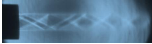
(b) Nozzle controlled with 2.5 mm strut
