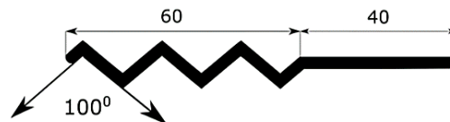
Fig. 3. Geometry of the Fruit Fly wing Cross Section (All dimensions are in mm).
