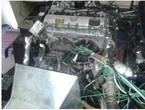
Fig. 7. Turbocharged engine on the test bench during the experiments (courtesy of IPCO).
