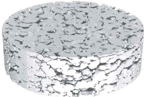
Fig. 1: CAD Model Generated from Scan of Mixing-disc
