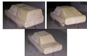
Fig. 3. The test models located on the six-component balance
