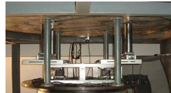
Fig. 2. Floating-frame strain gauge six-component balance
