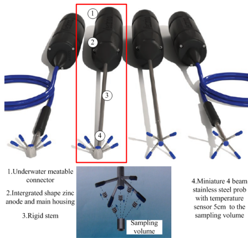
Fig. 2. The structure of the side-looking ADV and the sampling volume working principle. From the user guide of Nortek, 2004.
