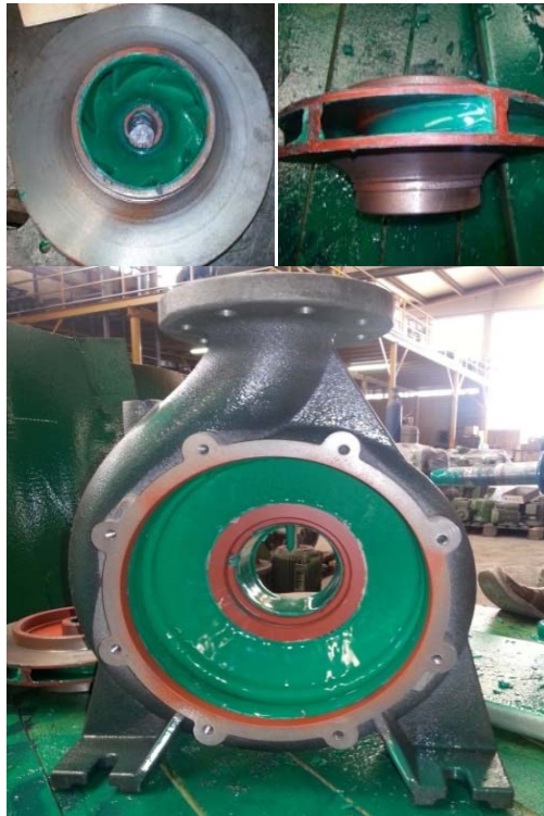
Fig. 5. Photographs of polyurethane coating process.
