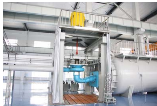
Fig. 1. The test rig of the pump-turbine model.
