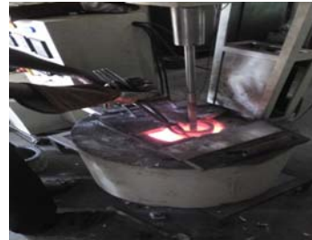
Fig. 1. Stirring of molten metal in the furnace
