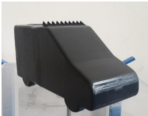
Fig. 7. Vortex generator application on model 1 (experimental).
