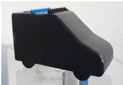
Fig. 8. Vortex generator application on model 2 (experimental).
