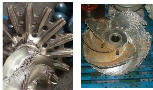
Fig. 1. Blade surface subjected to cavitation erosion
