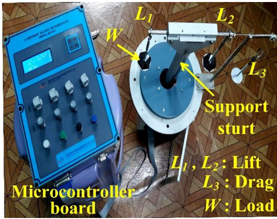
Fig. 6 Calibration setup for force balance
