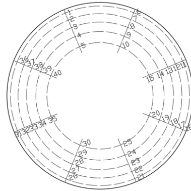
Fig. 2 Schematic diagram: (a) five-hole total pressure probe and (b) outlet total pressure measuring point layout
