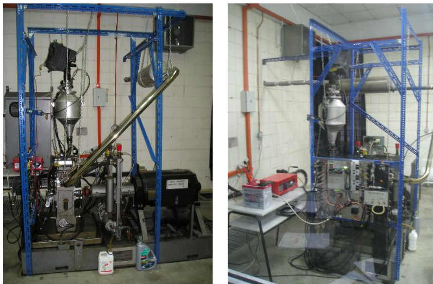
Fig. 29. The SCRE test rig of CNG-DI engine.
