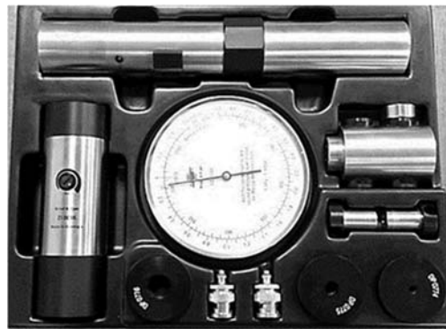
Fig. 4. Brüel and Kjær Type 3541 sound calibrator.
