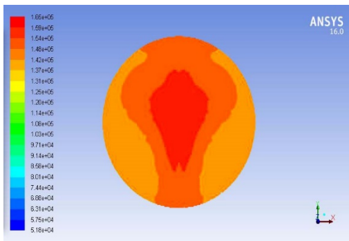
Fig. 7b. Pressure contour at Intake duct exit plane at M # 0.8, AoA=0°
