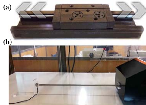
Fig. 9. a) Rail and wagon mechanism and; b) Load cell mechanism to measure drag force.
