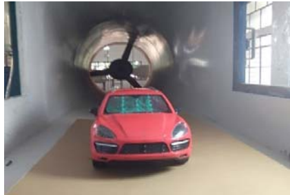
Fig. 3b. Car model mounted in the wind tunnel
