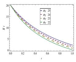
Fig. 7. Effect of  $R_T$  on depth for Ellis fluid,
