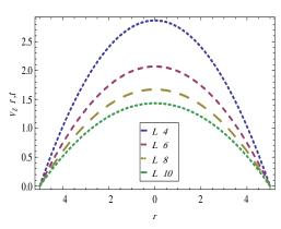
Fig. 5. Difference of L on the velocity profile for Ellis fluid, when  $\alpha = 1, \rho = 0.78 \text{ g/cm}^3$ ,
