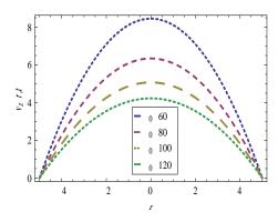
Fig. 3. Effect of  $\eta_0$  on velocity profile for Ellis fluid, when  $\alpha = 1$  poise,  $\rho = 1.38$  g/cm<sup>3</sup>, R = 5 cm,  $S_{\frac{1}{2}} = 21.554$  dyn/cm<sup>2</sup>,
