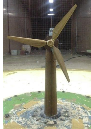
Fig. 1(b). Experimental pressure model with tower and rotor case
