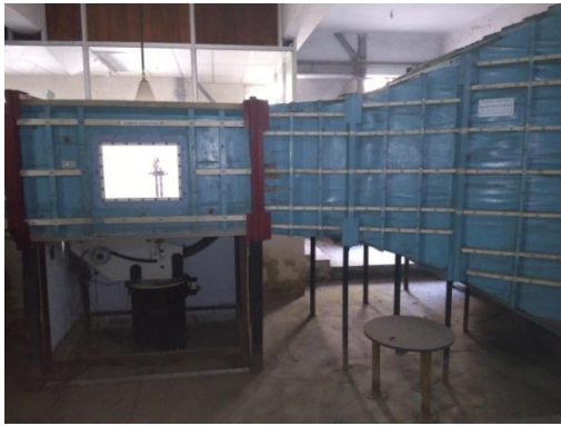
Fig. 2b. Open type sub-sonic wind tunnel.
