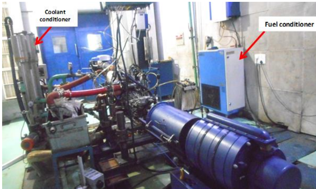
Fig. 2. Test engine setup with instrumentation.
