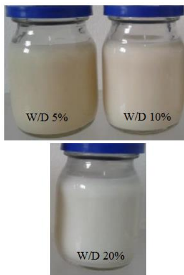
(b) W/D Emulsion samples with 5%, 10%, 15%, 20%, and 25% water
