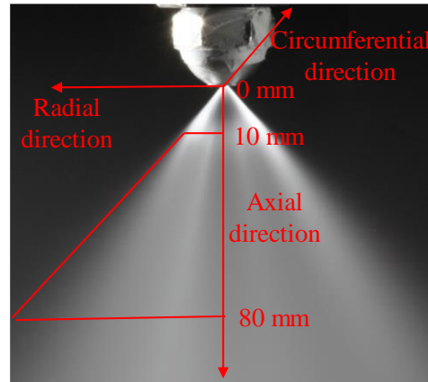
Fig. 12. Schematic diagram of measurement area.
