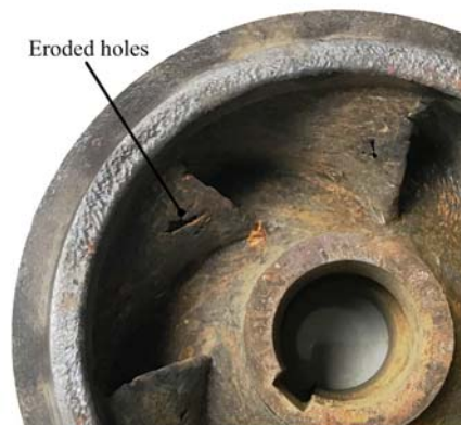
Fig. 3. Eroded impeller with holes after running 7000 h.
