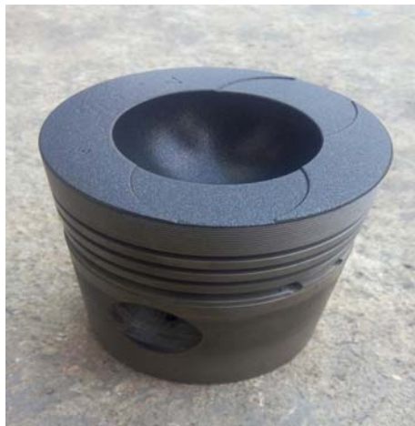
Fig. 2. Snapshots of uncoated piston and mixture of YSZ and MgO – TiO 2 coated piston.
