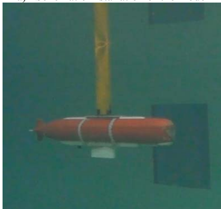
b) Image of model installation in underwater test
