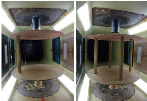
Fig. 7. Force-measured device of single conductor and quad bundle conductor.
