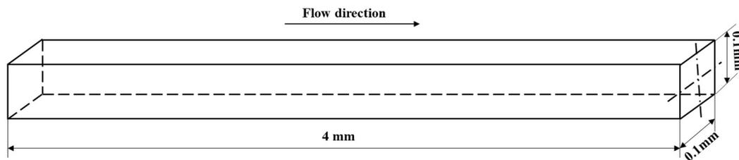
Fig. 1. Schematic of the 3D microchannel (AR = 1).
