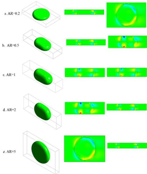
**Fig. 10. Droplet shapes and the radial velocity contours in a microchannel with different aspect ratios.**
