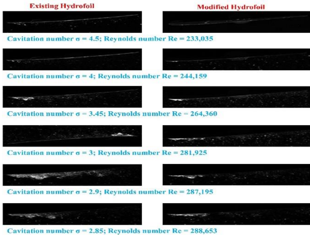
Fig. 15 Cavitation structures at P_{abs}=0.45 bar
