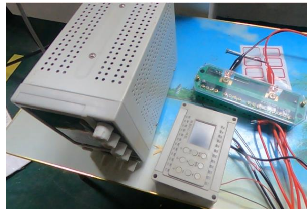
Fig. 6 Launch timing control module
