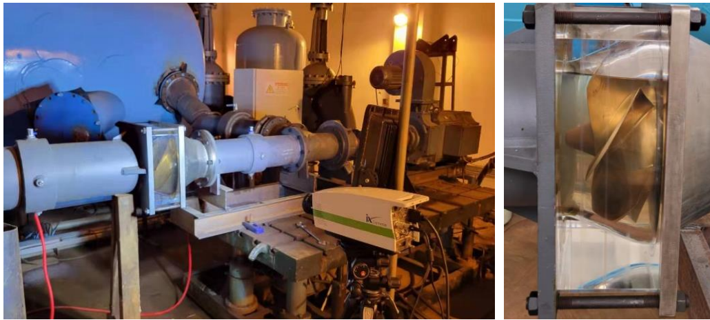
Fig. 4 High-speed photography visualization experiment system
