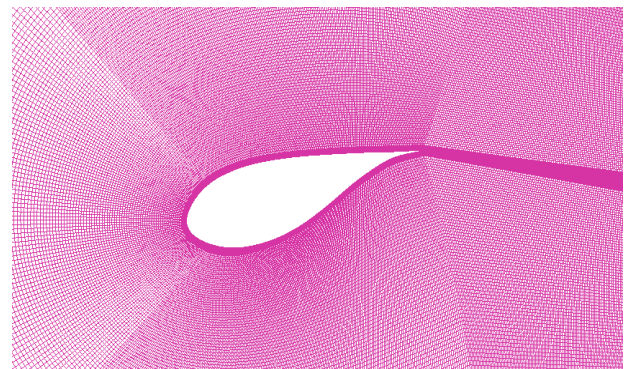
Fig. 3 Grid around the blade at root section
