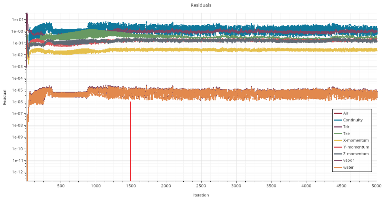
Fig. 13 The residual of the CFD equations solved at an inlet velocity of 3.5 m/s
