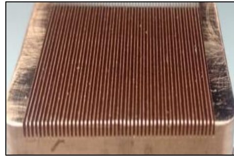
44 parallel Copper Microchannels w = 200 \mu\text{m}, d = 500 \mu\text{m}
