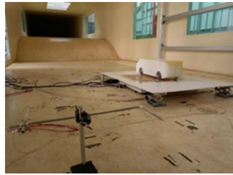
(a) Test model installed in the wind tunnel
