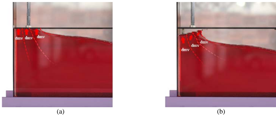
Fig. 9. Procedure of liquid collision to the flat and stepped roof types.
