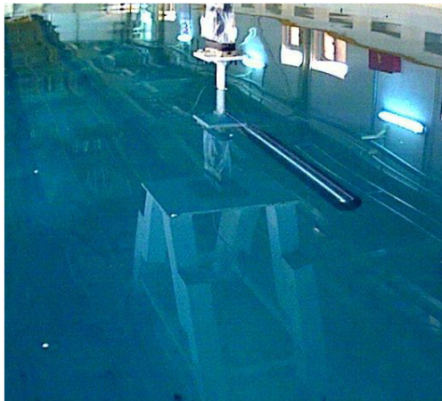
Fig. 7. Underwater hydrodynamic model associated with pylon in the towing tank laboratory
